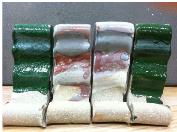
FIGURE 6b. Tiles 5 – 8, from left: Florentine green stain, combined copper and cobalt carbonates, combined lavender stain and copper and cobalt carbonates, combined rutile and Florentine green stain. Glaze applied over black and white slip on each tile.
